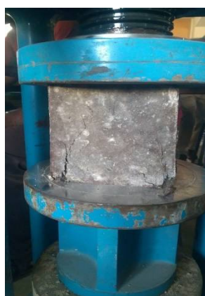
Fig No: 1 Compressive strength test
