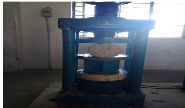
Fig No:2 Split Tensile strength test
