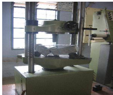
Fig No:3 Flexural strength test
